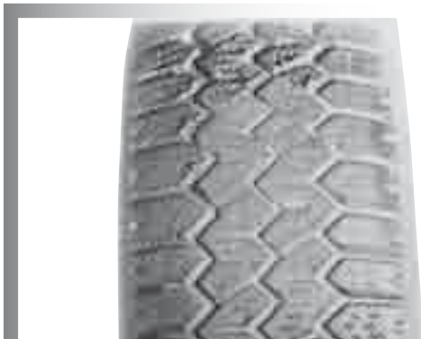
Severe wear due to full braking (without ABS).
