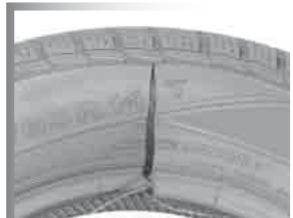
Ruptured bead as a result of tension during inflation of a tyre.
