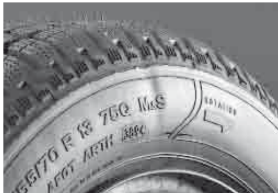
Indentation at the carcass ply overlap seam.
