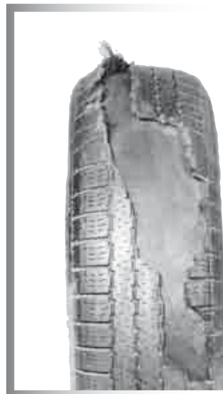
Parts of the tyre have torn off as a result of poor maintenance.
