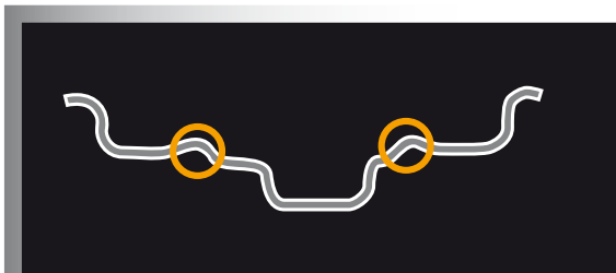
Rim profile with round hump on both sides (H2).
